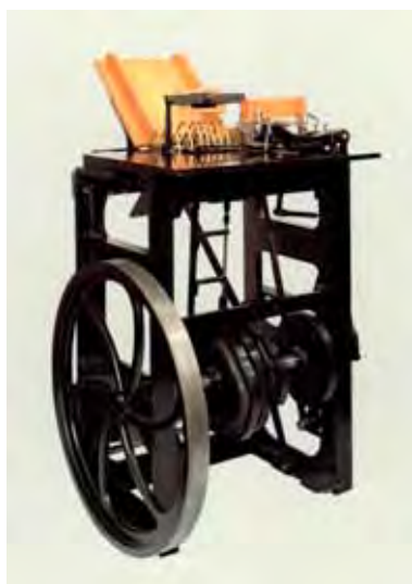
Fig. 1 The treadle-operated first field tested Pearson Hill postmarking machine. Photo courtesy of the British Postal Museum & Archive.
